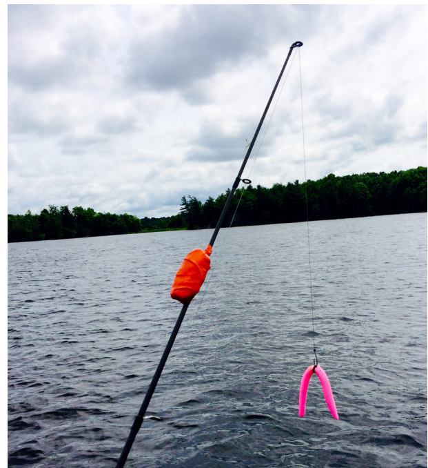
Figure 1: Fishing rod with tri-axial accelerometer attached for measurement of angling fight intensity.
